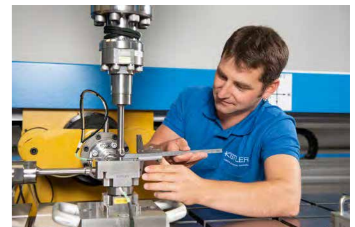
Multi-component force calibration: measuring of cylinder positions
